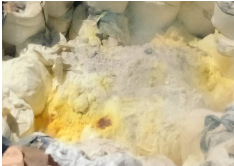
Moisture affected and decomposed sodium metabisulfite, having produced other yellow sulfur compounds.
