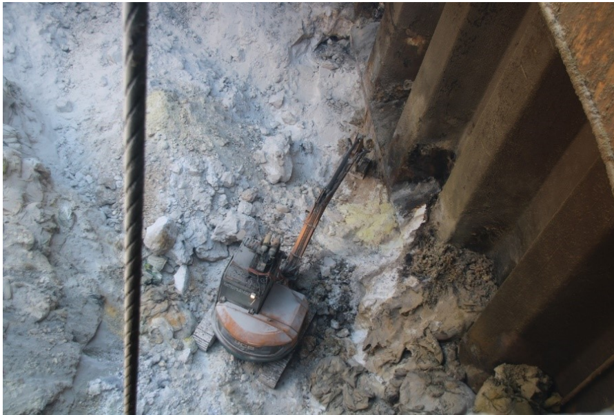
Operations to remove reacted cargo from a cargo hold (image taken from SAMSA website).
