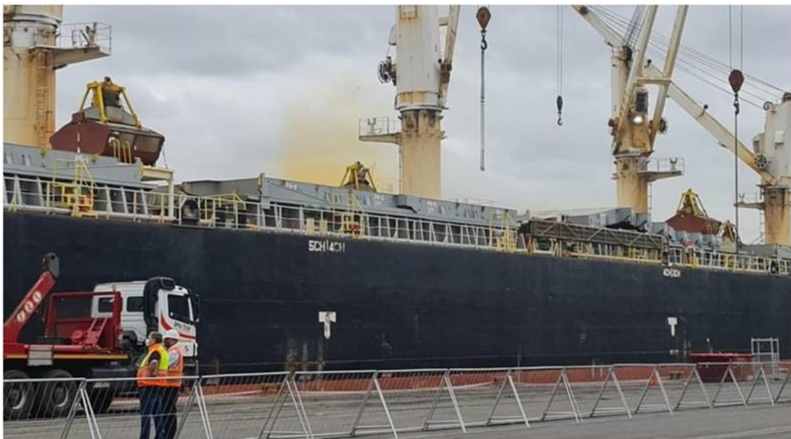
Toxic corrosive gases being released from a cargo hold containing a reacting cargo (image taken from South African Maritime Safety Authority (SAMSA) website).
