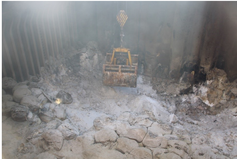
Operations to remove elevated temperature cargo from a cargo hold (image taken from SAMSA website).
