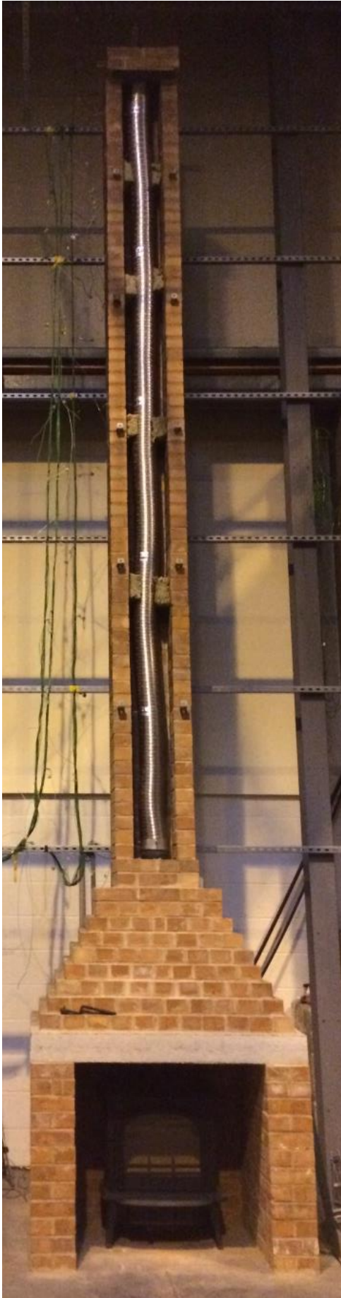
Figure 21 - Convection and Conduction mode test rig
