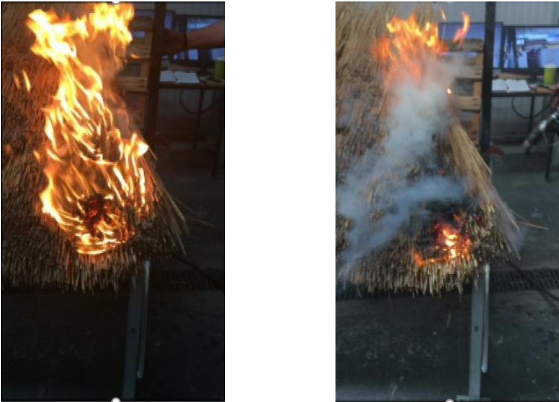
Figure 46 - Photo sequence of bird's nest test
