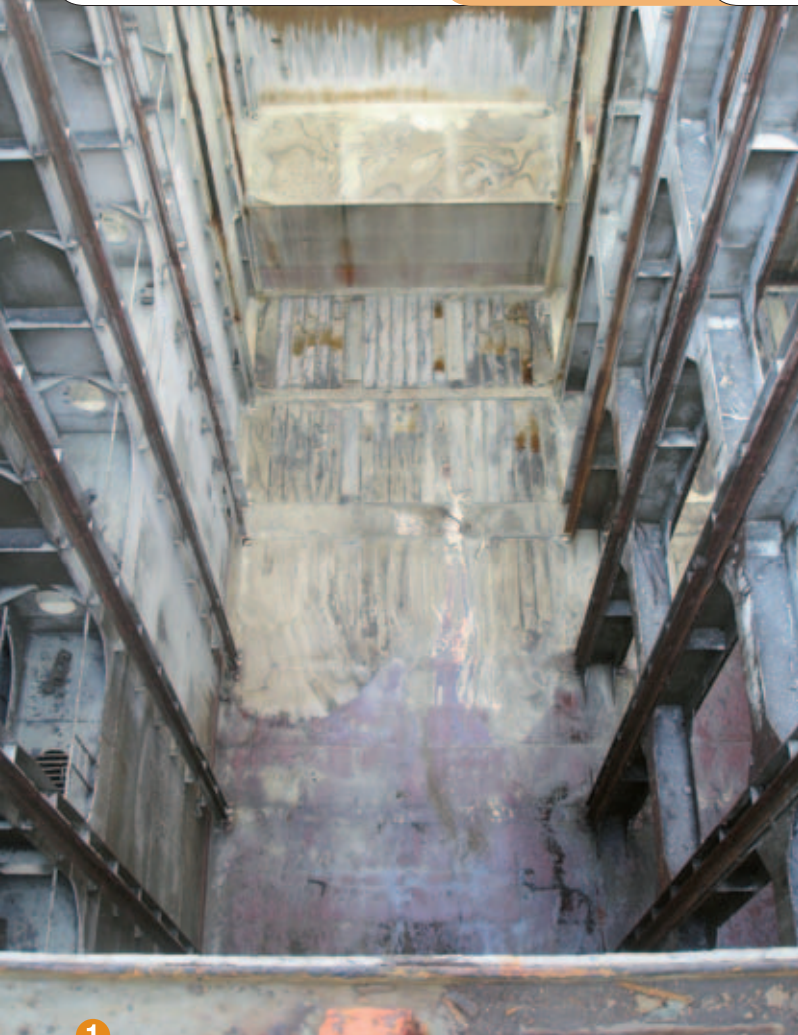
Widespread contamination of surrounding areas in the cargo hold.
